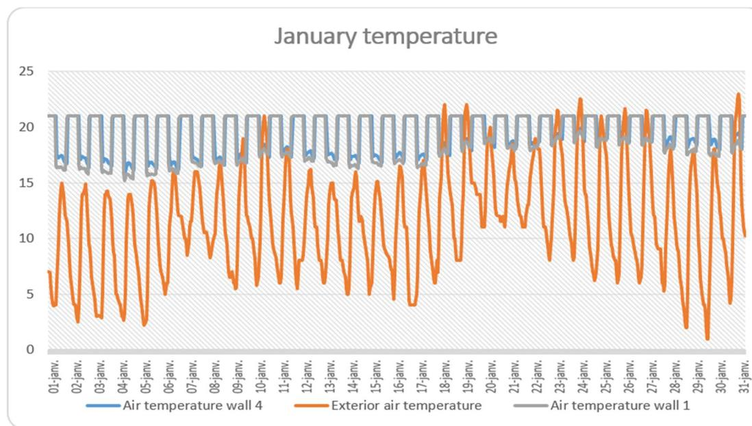
**Figure 12.** Temperature fluctuations (for wall 1 and wall 4) in typical months: (a) July, (b) January.
