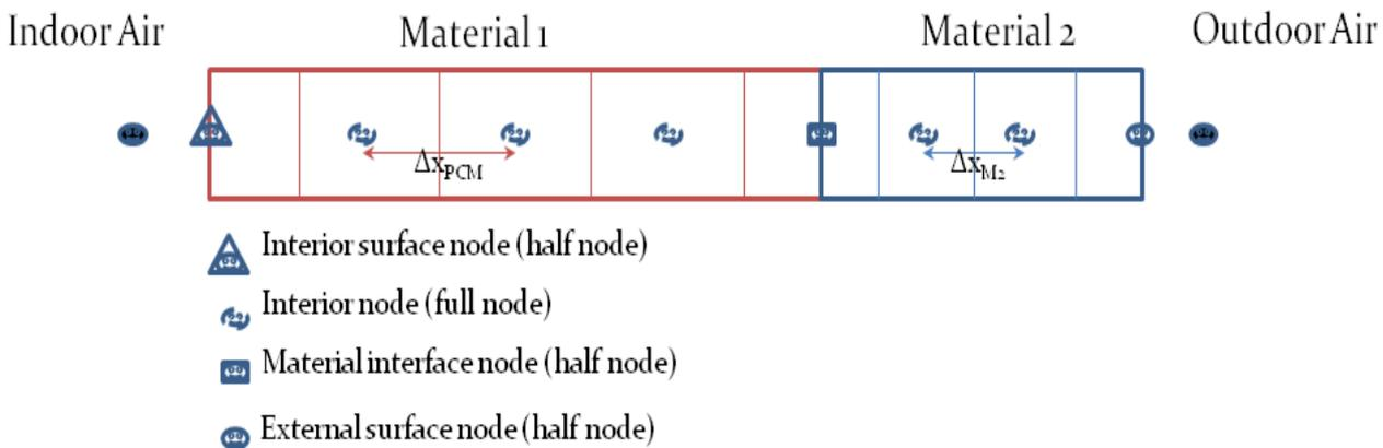
**Figure 6.** Node depiction for conduction finite difference method.
