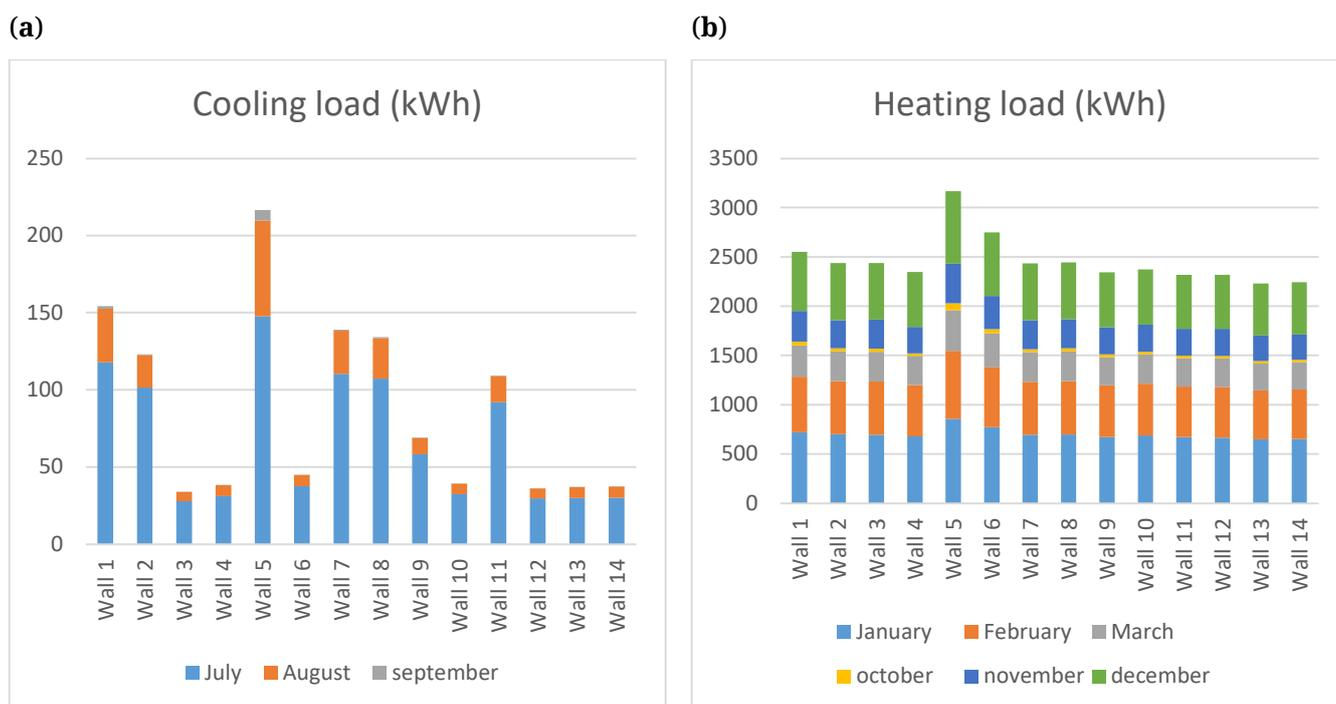
**Figure 10.** (a) Annual cooling load, (b) Annual heating load.
