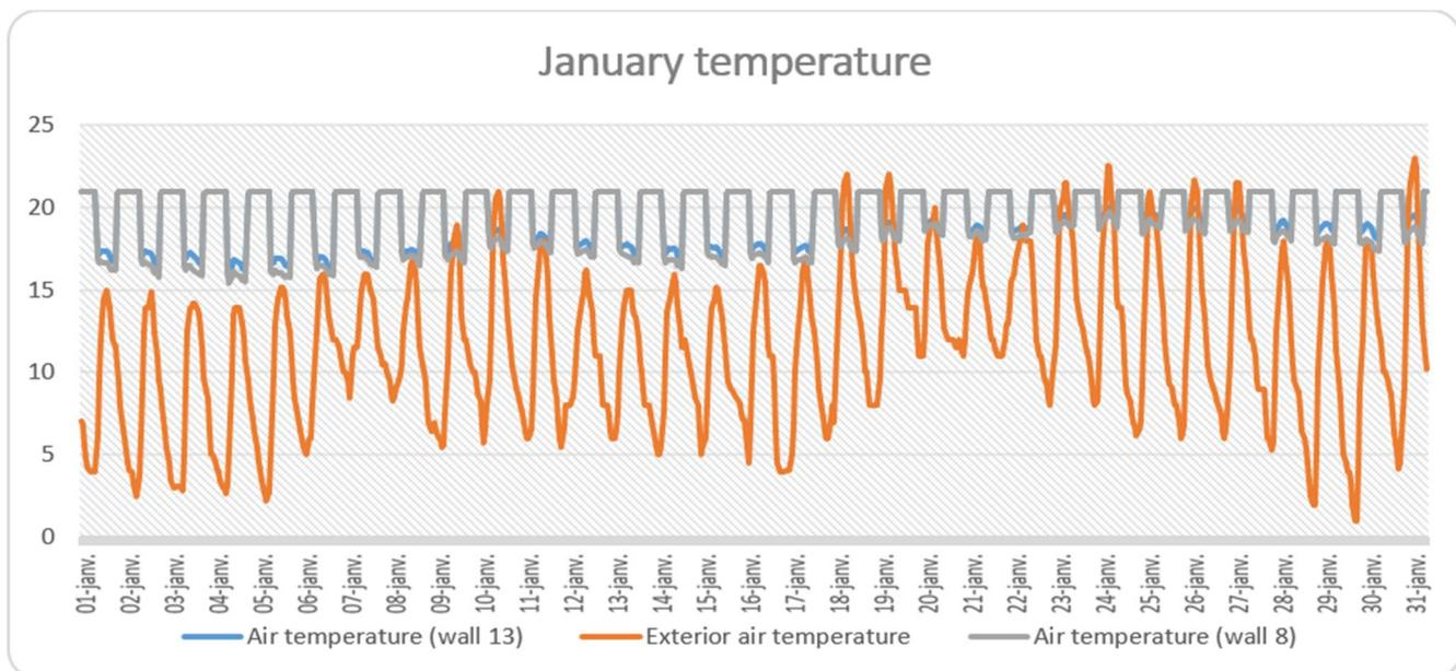
**Figure 13.** Temperature fluctuations (for wall 8 and wall 13) in typical months: (a) July, (b) January.
