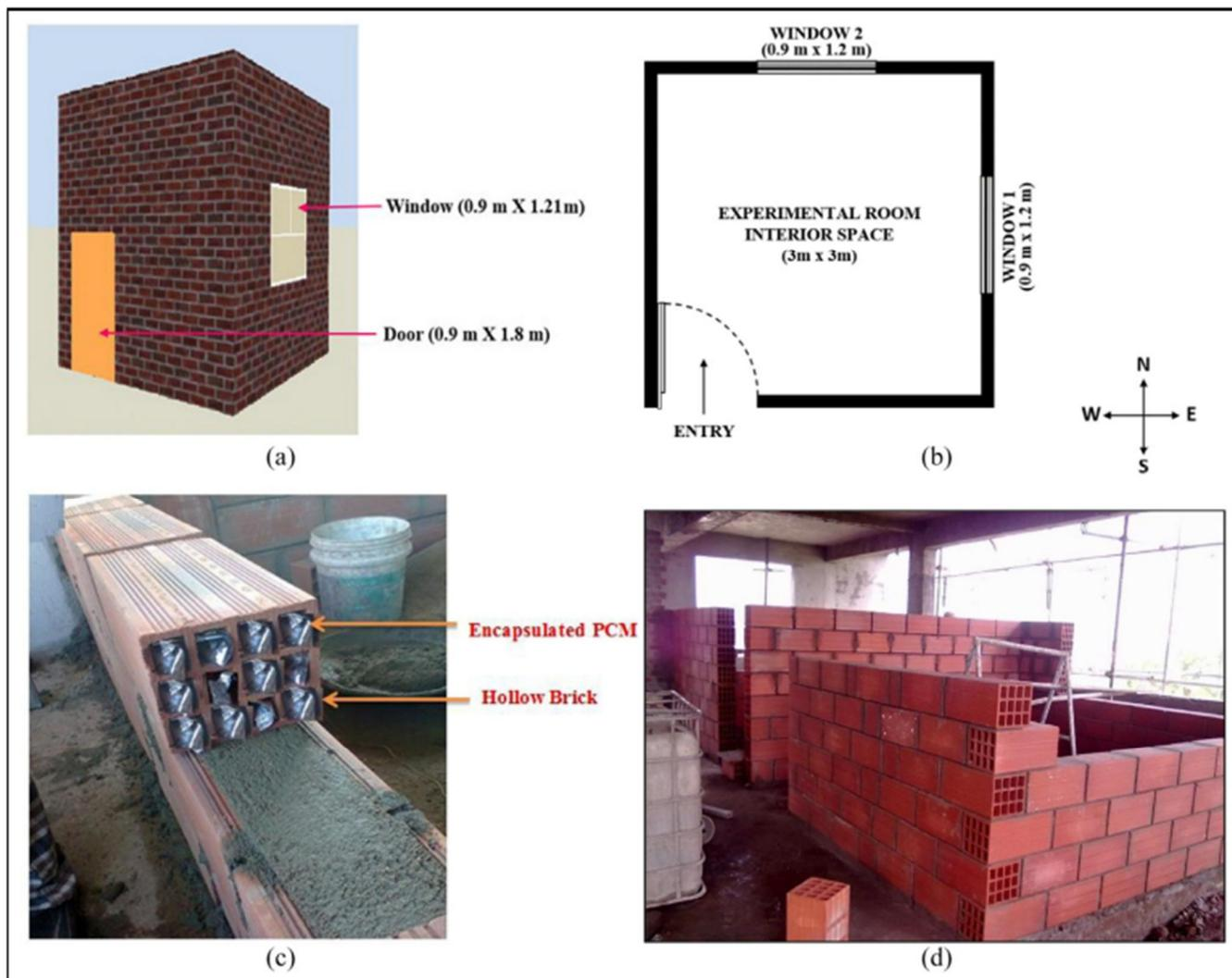
**Figure 7.** Description of the experimental setup.
