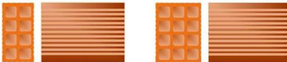
**Figure 4.** Two types of hollow brick wall, left: type1 (8 hollows) and right: type 2 (12 hollows).
