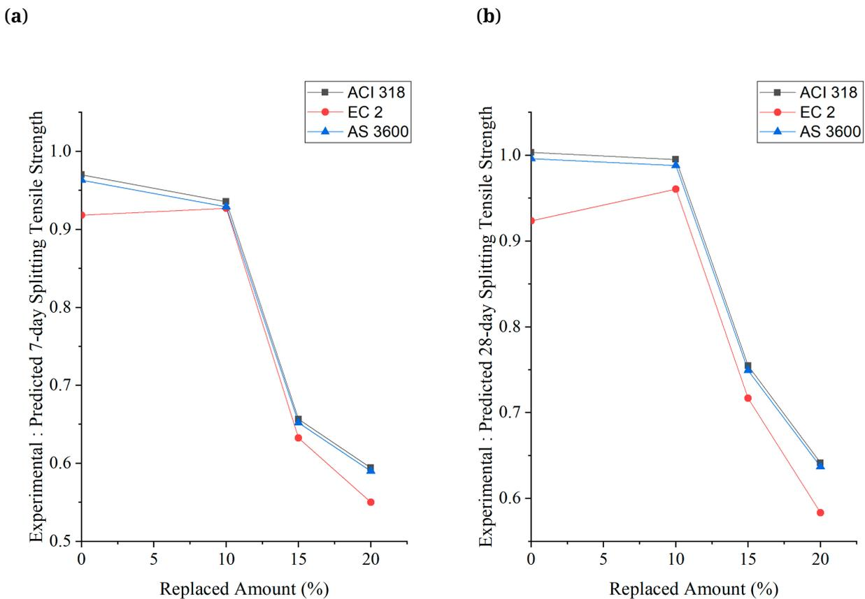
**Figure 12.** Variation of splitting tensile strength ratio at; (a) 7-day and (b) 28-day under different design codes.
