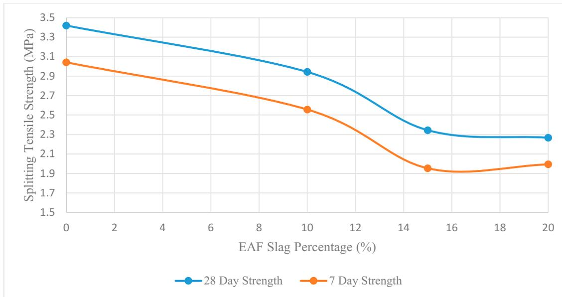
**Figure 9.** Variation of splitting tensile strength with EAF slag percentage.
