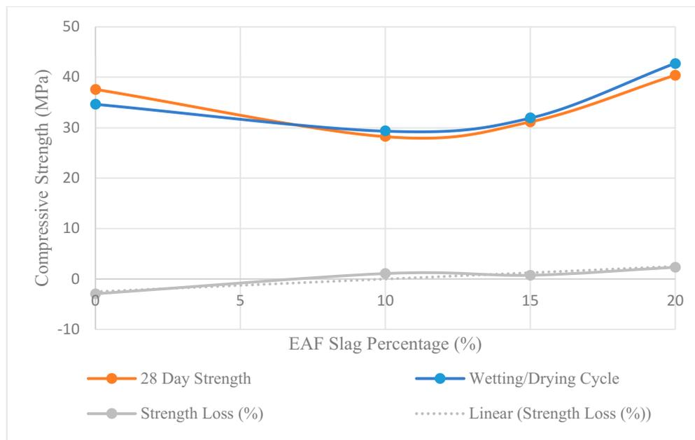
**Figure 8.** Average compressive strength variation before and after wetting/drying cycles.
