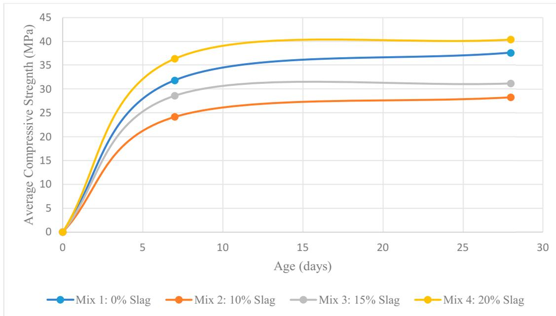
**Figure 6.** Average compressive strength variation with time.
