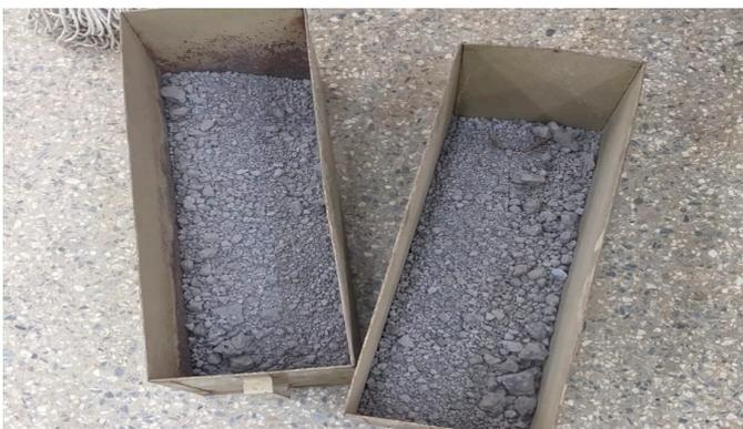
**Figure 1.** Sampling aggregates using riffle box.
