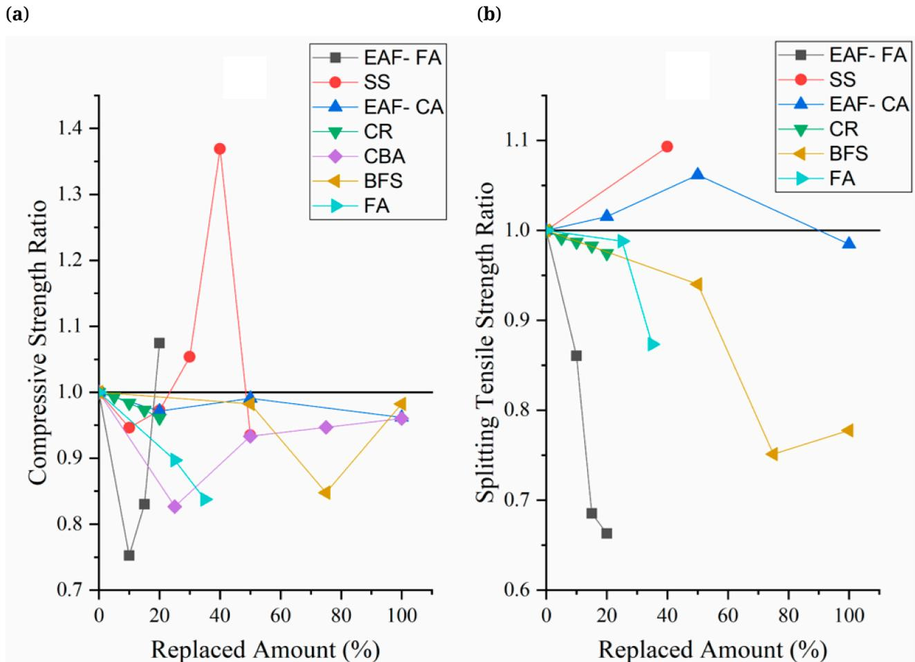
**Figure 11.** Influence of different materials to the 28-day; (a) compressive strength and (b) splitting tensile strength of concrete.
