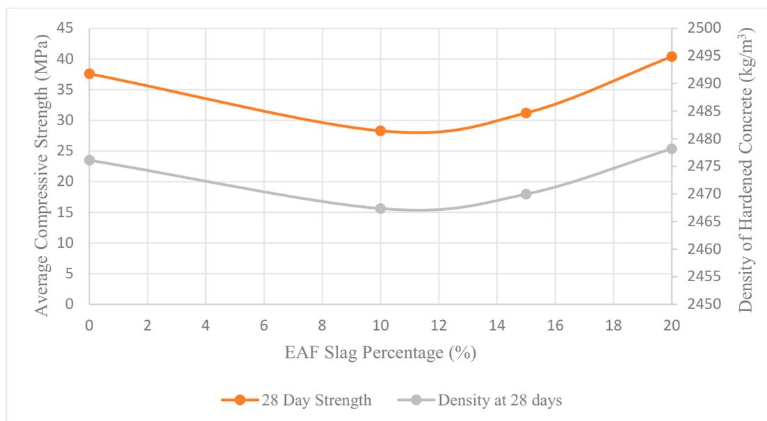
**Figure 7.** Comparison of average compressive strength and density at; (a) 7 days and (b) 28 days.
