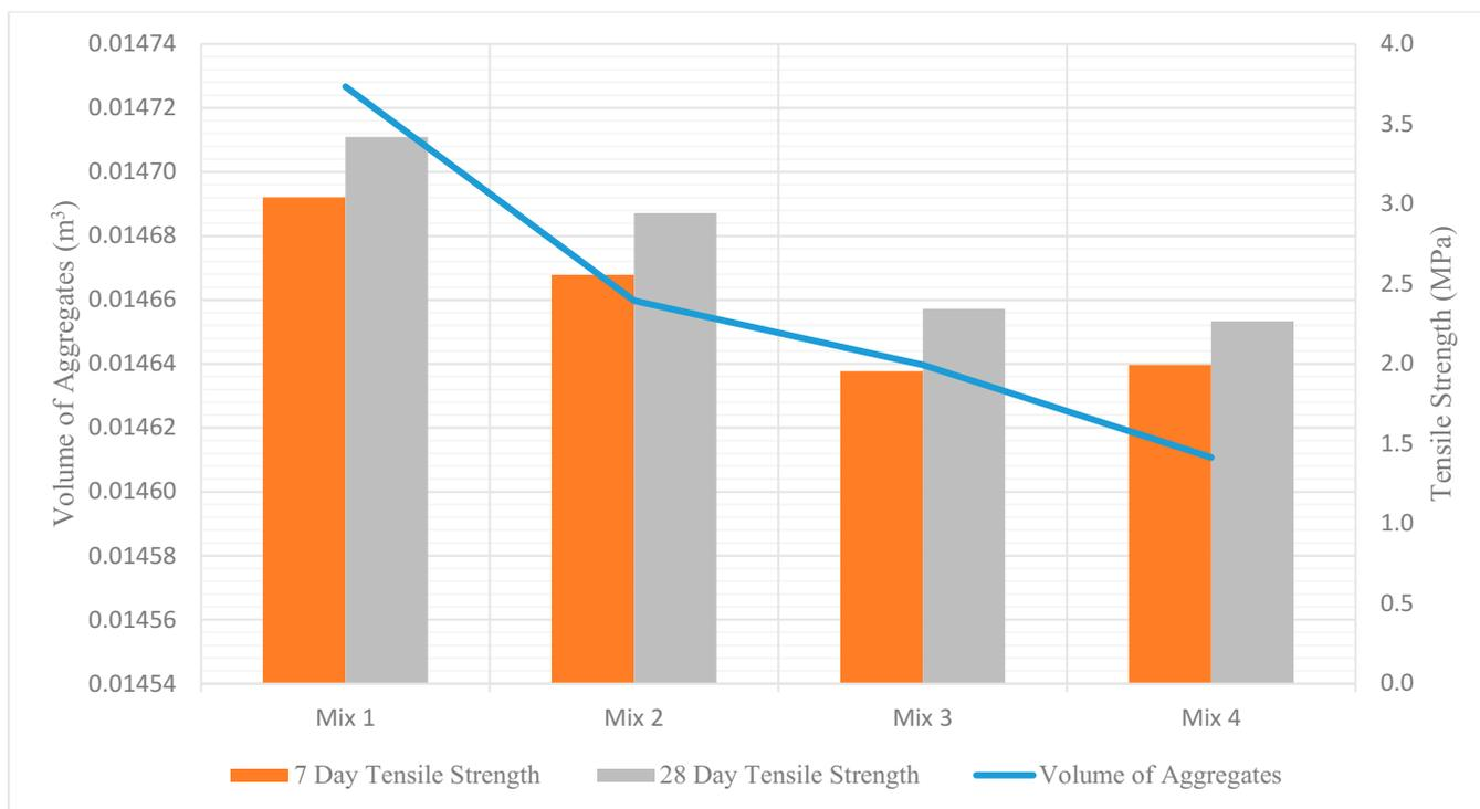
**Figure 10.** Comparison between volume of aggregates and tensile strength.
