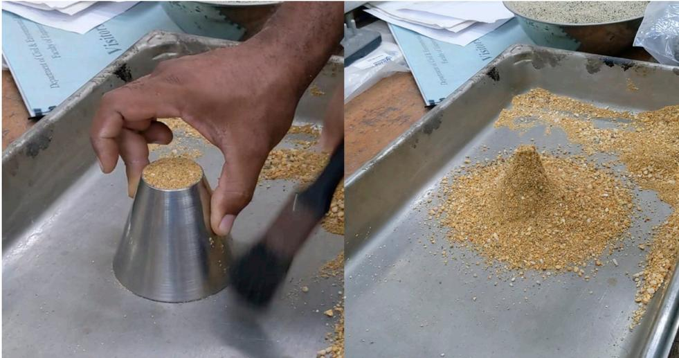
**Figure 3.** Slump test to determine if surface wet was achieved.
