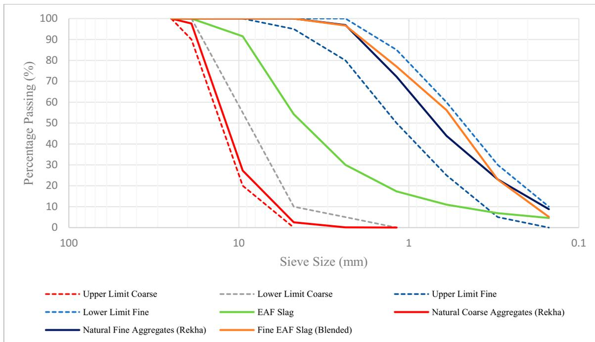
**Figure 2.** Particle size distribution of coarse and fine natural aggregates and electric arc furnace slag.
