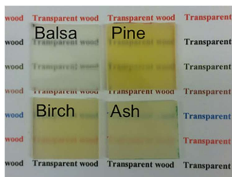
Figure 2. Transparent wood samples from four different species: Balsa, Pine, Birch, and Ash wood [16]. (Reprinted with permission from [16], Copyright the European Chemical Societies Publishing 2017).
