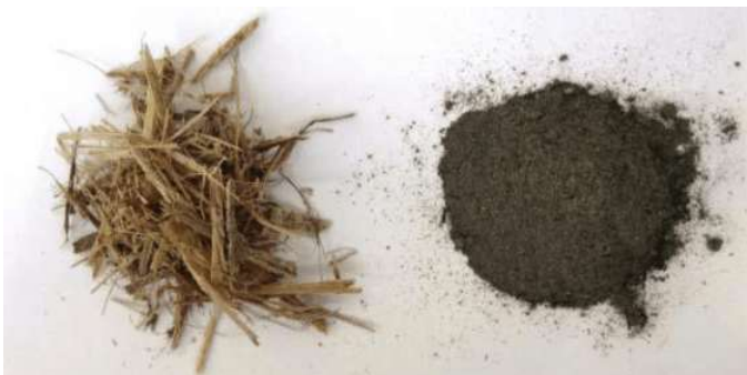
Figure 1. Visual comparison between raw sugarcane bagasse ( left ) and SCBA ( right ), illustrating the transformation of an agro-industrial residue into a silica-rich byproduct with potential application as a supplementary cementitious material [36].
