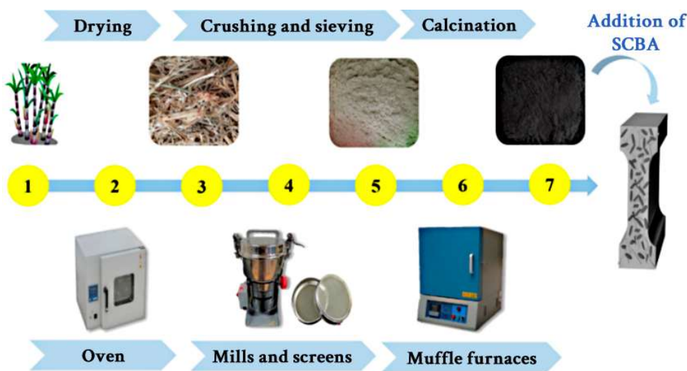
Figure 4. Typical process flow for SCBA preparation showing drying, crushing, calcination, and grinding steps [34].
