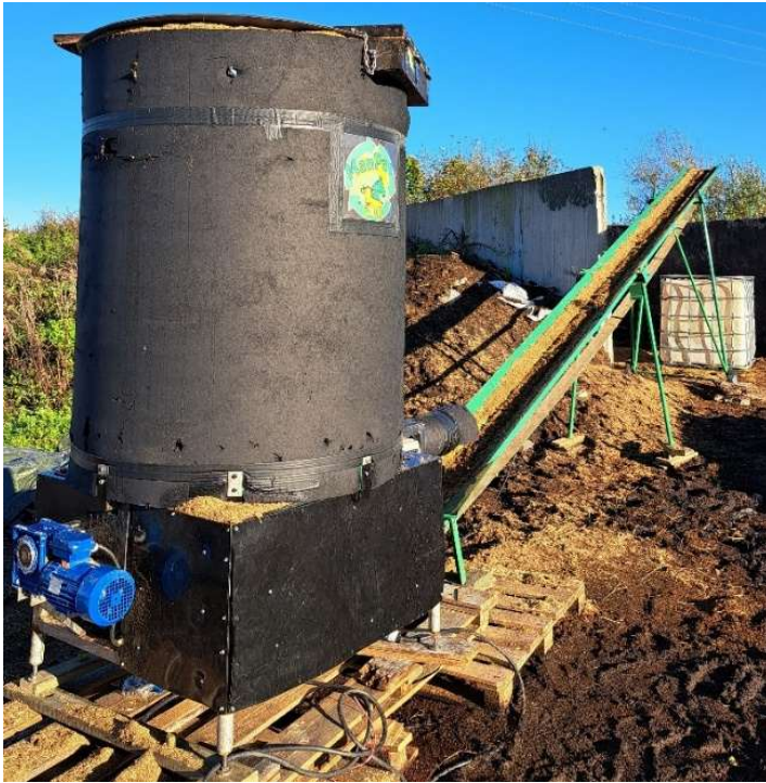
Figure 2. Test setup: a belt conveyor connected to the ManPas system that transfers manure from the screw to the IBC container.
