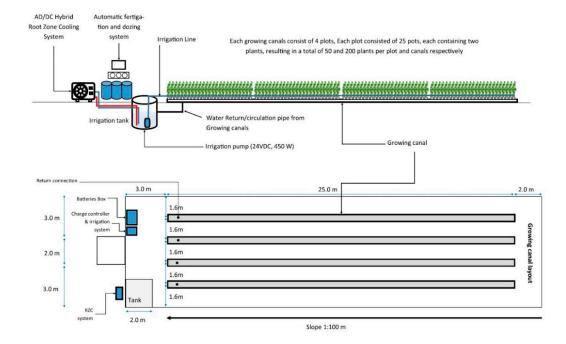
Figure 4. Study layout and setup under the net house in Oman and UAE.
