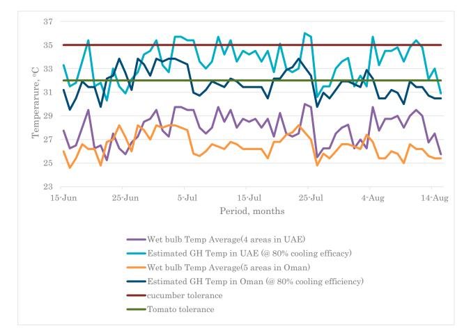
**Figure 1.** Average daily wet-bulb Temp in UAE (Abu Dhabi, Dubai, Fujairah and Al Ain) and Oman (Semail, Seeb, Al Merat, Muscat, and Ibra), between 15 June to 15 August 2022 and estimated greenhouse temperatures based on 80% efficiency of evaporative cooling system [9].
